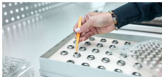
Preparation for the welding process: Placing the lenses on the stainless-steel sleeves is still manual work.
