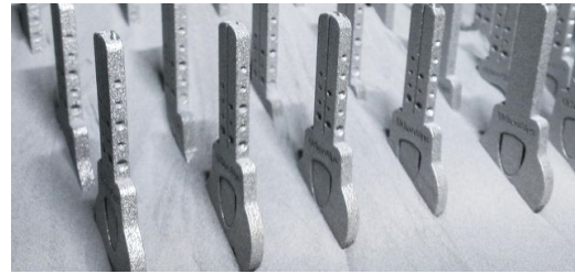
The 3D printing process enabled the young engineers to completely redesign the traditional key. Picture: UrbanAlps
