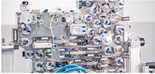
Mirror support on a EUV-module
