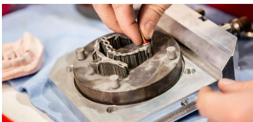
The telescopic crown is built up layer by layer from the powder bed. After this step, the crowns match the geometry of the primary coping almost perfectly, apart from a minimal amount that has to be milled off the inner surfaces. (Picture: Steffen Müller-Klenk)
