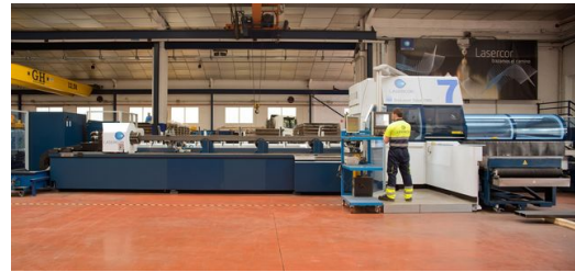
In addition to 2D laser cutting, bending and engraving services Lasercor is specialised in laser tube cutting. The company processes a range of materials, including structural and stainless steel, aluminum, brass and copper. (Pototo Diez)
