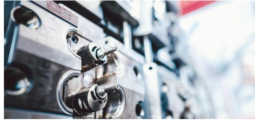
The challenge lay in this injection mold for the brush holder. The part poking out is the steel pin made using LMF and LMD. (Picture: Philipp Reinhard)
