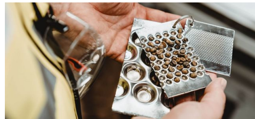
A perfect fit: The dot marking must fit exactly into the depressions in the sheet, the "pockets".
