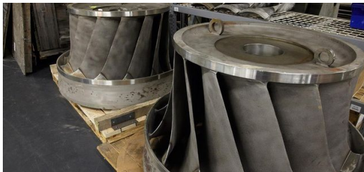
Laser-cladded turbines: "Does it work?" is a question Dan Hayden often hears. Photo: Steve Adams Photography
