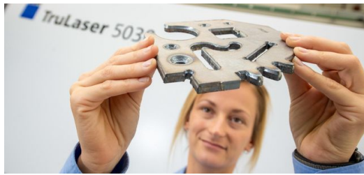
<p><span lang="EN-US">A worker checks a component she has chamfered using TRUMPF's EdgeLine Bevel technology. </span></p> – TRUMPF / Martin Stollberg
