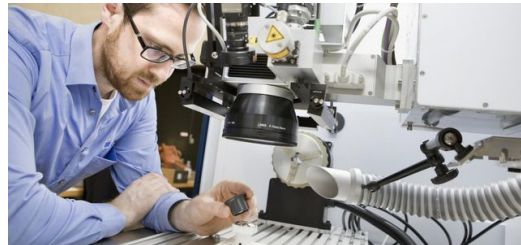
For the engraving of the platinum watch backs, TRUMPF machine operator Matthias Widmer very carefully approached the desired engraving depth of 17 micrometers.
