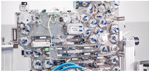
Mirror support on a EUV-module
