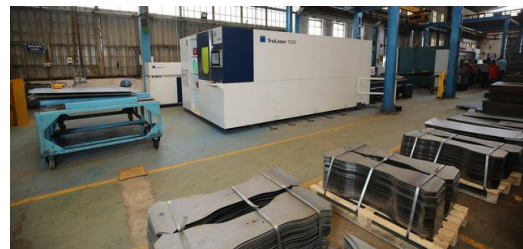
JBM has been using the TruLaser 1030 laser machines for sheet metal cutting for several years.
