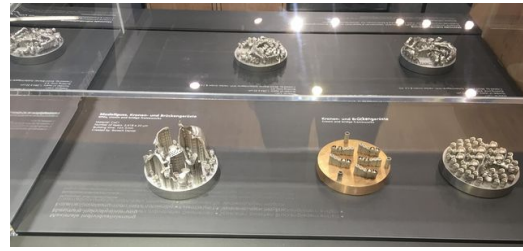
<p>Substrate plates with 3D-printed dental prosthesis.</p>
