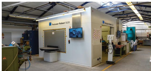
<p>Hey Mr. Robot: The TruLaser Robot 5020 helps Gefinal perform challenging welding jobs.</p> – Christian Mader
