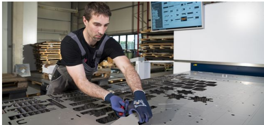
Today, all it takes is a glance at the Sorting Guide screen. The operator is shown a removal proposal on the large screen. All parts that belong to an order are color-coded.
