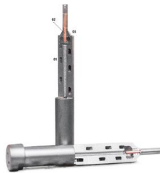
Two additive methods are used to produce the metal pin in the mold: the 3D-printed steel body features cooling channels (1) and contains a fast-cooling copper pin (2) which is built up in layers using LMD and joined to the steel body (3). (Picture: Philipp Reinhard)
