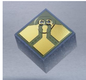
Chip die – two 850 nm VCSELs with single integrated photodiode (ViP) for high-volume self-mixing interferometry sensing applications and integrated speed sensors
