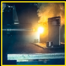
Tests show that the laser cutter also works well underwater.
