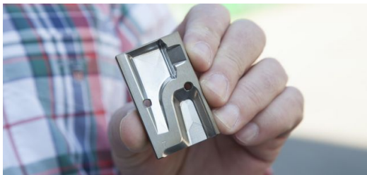
The molded gripper forces the blanks into a defined position, aligning them with the laser machine’s reference system.
