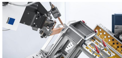
The FusionLine joining technique can be used to join parts, even when this involves the bridging of gaps. It smooths out any unevenness during the welding process and closes gaps up to one millimeter wide. That makes it possible to use the laser on many parts that were originally designed for conventional welding methods. (Picture: Oliver Graf Fotostudio GmbH)
