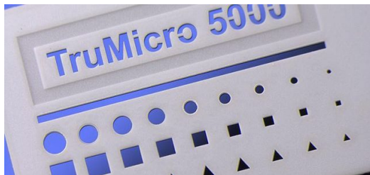
With regard to bezels and watch casings made of ceramic: no tool other than an ultrashort laser beam can create contours like these with such speed and precision. Picture: TRUMPF
