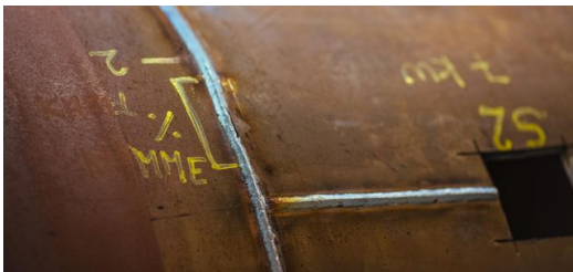
Welds up to 25 millimeters deep: Force Technology /LWT engineers use a 32-kilowatt laser to demonstrate laser hybrid welding processes for the maritime and the offshore wind turbine industries. Photo: Kasper Fladnose
