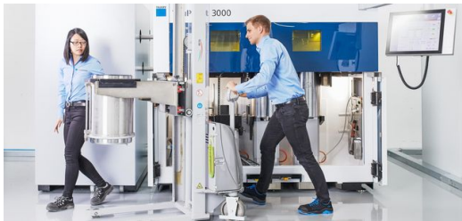
Removing the cylinder containing the part from the 3D printer. The part is now ready for further processing.
