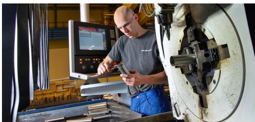
<p>Each day one or two of the programmers are fully occupied with preparations for two-shift operations. The TruTops Tube Software makes possible exact calculation of cutting geometries. Picture: Escherich Fotografie</p>
