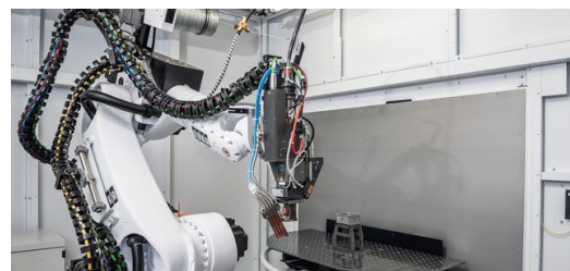
The laser network, serving a TruLaser 3030 fiber and a TruLaser Robot 5020, expands the range of services offered by SCS by adding laser cutting and welding. Picture: Peter Oppenländer
