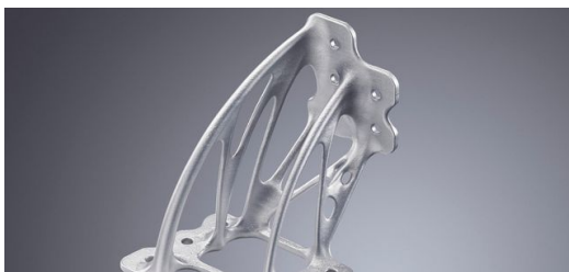
Lightweight construction: Weight reduced mounting brackets are particularly beneficial in aircraft construction. Here material is only accumulated along lines of force transmission.
