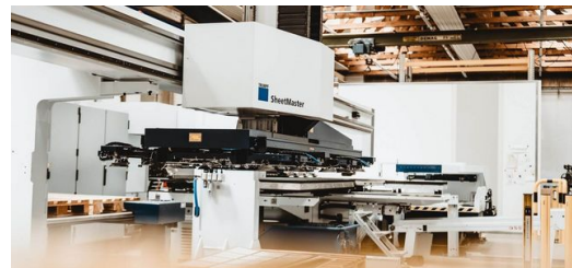
Automation: The SheetMaster supplies the TruPunch 5000 with the required material. This increases efficiency and takes the pressure off employees.
