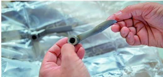
<p>All one piece: Redesigned by Bionic Production, this nozzle offers gentle curves straight from the 3D printer. Picture: Claus Langer</p>
