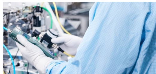
Light from CO 2 lasers requires a vacuum. Leak tests are performed to ensure that no air from the outside penetrates the system.
