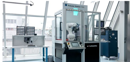
Efficient duo: At the Widnau site in Switzerland, endoscope manufacturer Karl Storz welds eyepieces on a TruLaser Station 7000. A mobile robotic cell takes care of loading and unloading the components.
