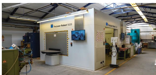
Hey Mr. Robot: The TruLaser Robot 5020 helps Gefinal perform challenging welding jobs.
