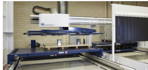
The SheetMaster is entrusted with loading and unloading the machine. It sorts the parts and lays them on the cart or pallet. (Picture: Claus Langer)
