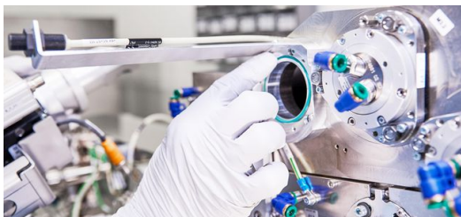
A mechatronics engineer installs a mirror mounting.
