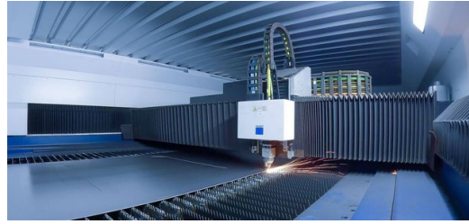
The laser head whizzes over the seemingly endless sheet metal strip and cuts the contours of the outer surface parts of the Fendt tractors.
