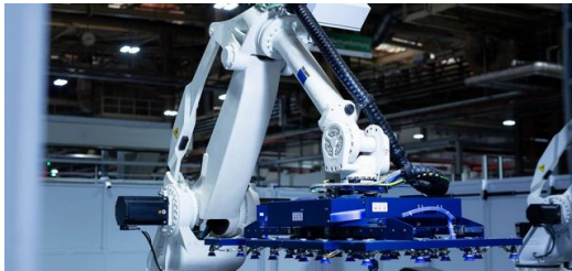
The two unloading robots have their work cut out for them: The components come out of the laser cutting chamber in streams.
