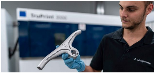
The handlebars are essentially based on a unit with semi-internal ducts for the brake cables.
