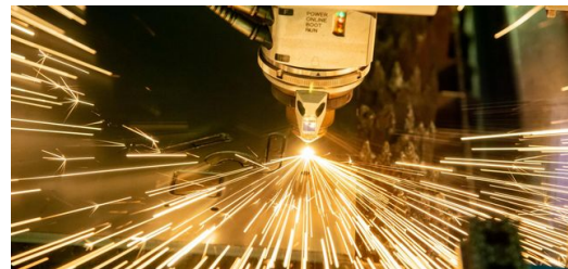
With EdgeLine Bevel technology, a TRUMPF standard machine for laser cutting produces beveled cutting edges on the contours of the component.
