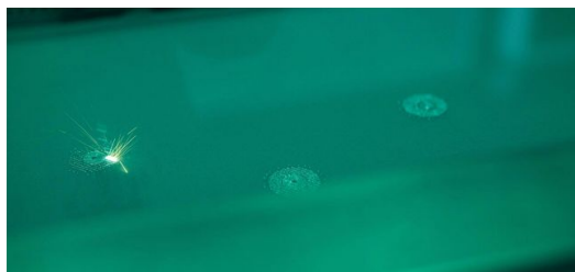
<p>Lasers are also used at Aesculap for the additive manufacturing of acetabular cups, among other things.</p>
