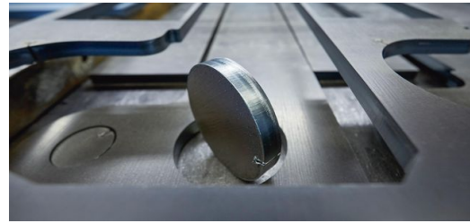
The BrightLine fiber option produces amazing cut edges at impressive speed, when working with mild steel 25 millimeters thick. (Picture: Claus Langer)
