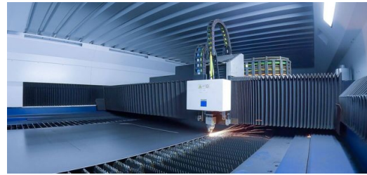
<p class="MAGAFIetext">The laser head whizzes over the seemingly endless sheet metal strip and cuts the contours of the outer surface parts of the Fendt tractors.</p>
