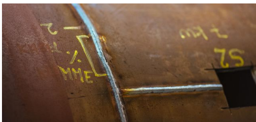
Welds up to 25 millimeters deep: Force Technology /LWT engineers use a 32-kilowatt laser to demonstrate laser hybrid welding processes for the maritime and the offshore wind turbine industries. Photo: Kasper Fladmose
