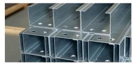
recise product analyses by the SCHRAG project group show that some profiles exhibit a certain degree of standardization. In the future, these profiles will be produced automatically on a roll forming line at SCHRAG's Hamburg Seevetal site.
