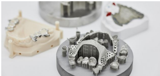
<p>Dentures from the TruPrint 1000 3D printer from TRUMPF.</p>
