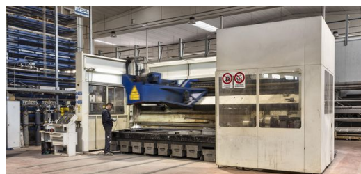
Multi-talented: ELFIM does not just use the Laser cell 1005 to weld and cut 2D and 3D components. The system is also suitable for laser metal deposition.
