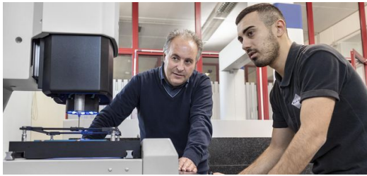
Replacement parts for classic cars are rare. Using the LMD process, they can be reconstructed in a cost-effective way. In such cases experts at ELFIM perform a 3D scan of an existing replacement part.
