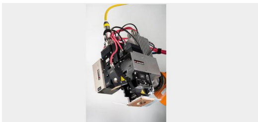
The laser processing optics system designed using modules supplied by specialist manufacturer Sansonic is equipped with a highly dynamic 1D scanner unit capable of generating variable track widths, and is compatible with industrial-scale production. Picture: Daimler AG
