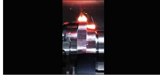
A too high laser output presents the risk of overheating and thus melting especially the finer edges and contour steps. Picture: Daimler AG
