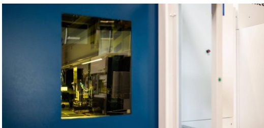
Laser-safe windows can usually be identified by their green color. In addition to a CE marking, a laser-safe window comes with further information, for example, on the protection level.
