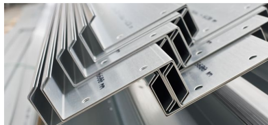
Typical order volumes at Schrag range from a single item up to batches weighing 20 tons. As well as top-quality, most customers also require very short turnaround times. The VarioPress 400 at Schrag has a higher-power motor and an additional height-adjustable axis that allows users to bend Z profiles. Picture: Dirk Egelkamp
