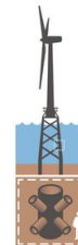
The nodes are a crucial part of the underwater lattice structure that supports a wind turbine. It takes several days to make one of these by hand - but the method developed by Force Technology / LWT gets the job done in just a few hours. Illustration: Gernot Walter
