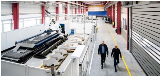
The 34 meter-long laser blanking system from TRUMPF saves unprocessed material and around 4000 tonnes of CO 2 per year.
