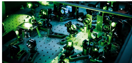
<p>L’Huillier’s research team in Lund, Sweden, uses femtosecond lasers to produce high-harmonic pulses of light. These are then used to generate attosecond laser pulses, which can render atomic processes visible.</p>
