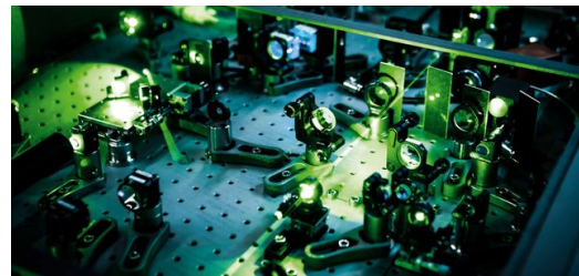
L’Huillier’s research team in Lund, Sweden, uses femtosecond lasers to produce high-harmonic pulses of light. These are then used to generate attosecond laser pulses, which can render atomic processes visible.
