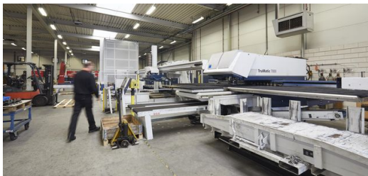
The company offers a high level of vertical integration. Bending and welding are just as much a part of the portfolio as laser cutting and punching - for example with the TruMatic 7000 punching laser machine (Photo: Claus Langer).
